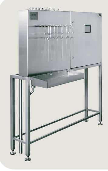
The sampling panel is connected via pipes of Ø10 mm to the pneumatic sample valves on the tanks. The connections can either be stainless steel pipes or Teflon hoses, with or without insulation, depending on local conditions.
