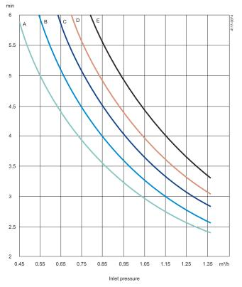
A = Nozzle: 1.18 mm Stator 3.5 B = Nozzle: 1.90 mm Stator 4.0 C = Nozzle: 2.03 mm Stator: 4.5 D = Nozzle: 2.16 mm Stator: 5.0
