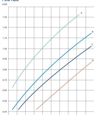
A = Nozzle: 2.16 mm Stator: 5.0 & 5.5 B = Nozzle: 2.03 mm Stator 4.5
