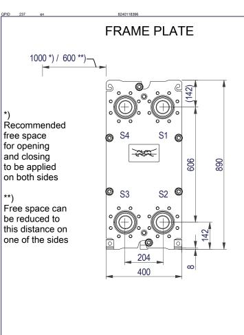
Space between pressure plate and supporting column should be kept free from fixed installations!
