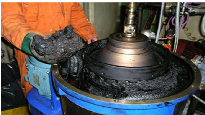
Figure 6: A separator subjected to instable fuel
