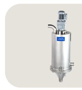
Any coarse particles suspended in the liquid are held back in the filter basket, and then forced downwards by rotating brushes mounted on a central shaft. This shaft is driven by an electrical gear motor mounted on top of the unit.
