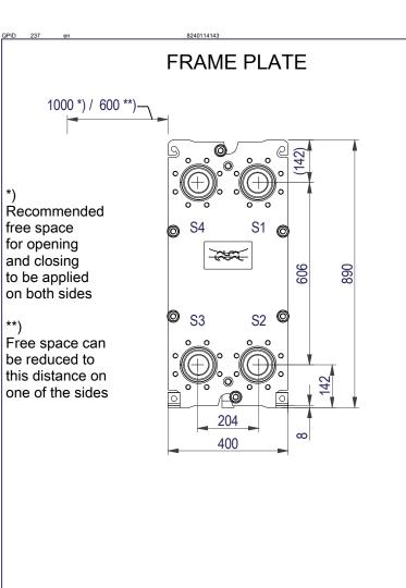
Space between pressure plate and supporting column should be kept free from fixed installations!
