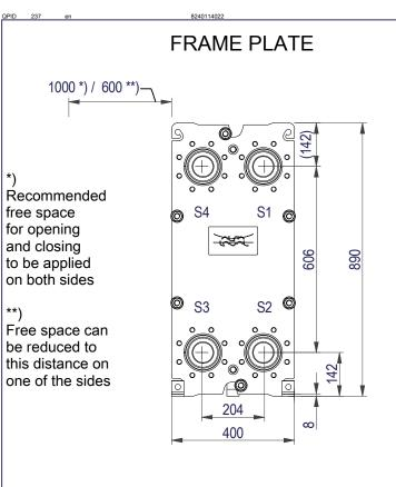
Space between pressure plate and supporting column should be kept free from fixed installations!
