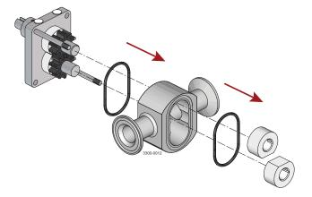
Remove the auxiliary shaft (22) with gear (20) and the rear bush (9) from the back plate (2).
