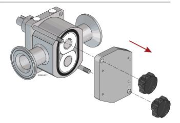
(4) Remove body (1) together with the Front and Rear body O-rings (5). **NOTE**: Front bushes (4) may stay in the body but can be removed by pushing out.
