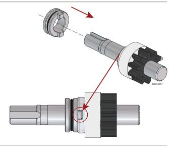
3 Fit O-ring (15) in the rotary seal ring (16) from the rear. Clean the rotary seal face with a suitable solvent and slide onto the shaft.
