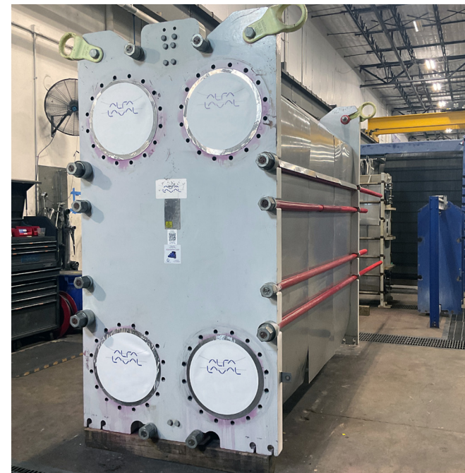
The reconditioned heat exchanger in Alfa Laval service center.
