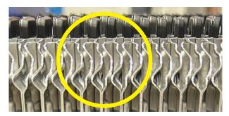
Asymmetric plates with asymmetric configuration will have the corners of the plates as in the image below. Two plates are close to each other and then there is a longer distance to the next pair of plates.
