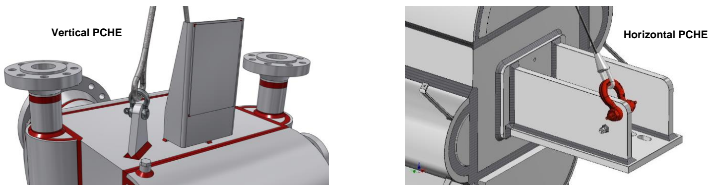
Figure 3. Dee-type shackles connected to lifting lugs for vertical unit (left) or horizontal unit (right).
