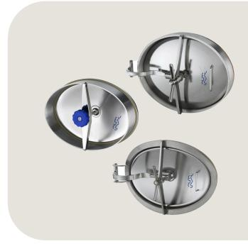
Alfa Laval Tank covers are available in AISI 304 or AISI 316L stainless steel. Surface finishes include electropolished lid and brushed frame and vary from Ra 0.8 to Ra 3.0. In addition, 3.1 Material Certifications in accordance with EN 10204 are supplied with the cover. For more information, please refer to documentation and the Tank cover selection guide (.pdf 1 250 KB).
