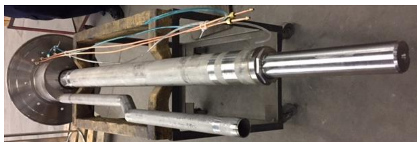
Figure 7.6-10: Remove drive line, bucket, lube & flush lines
