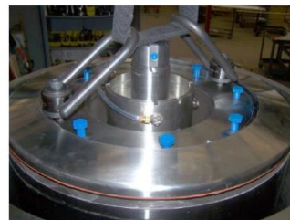
Figure 7.6-14: Attach the bucket assembly to the Contherm MAX
