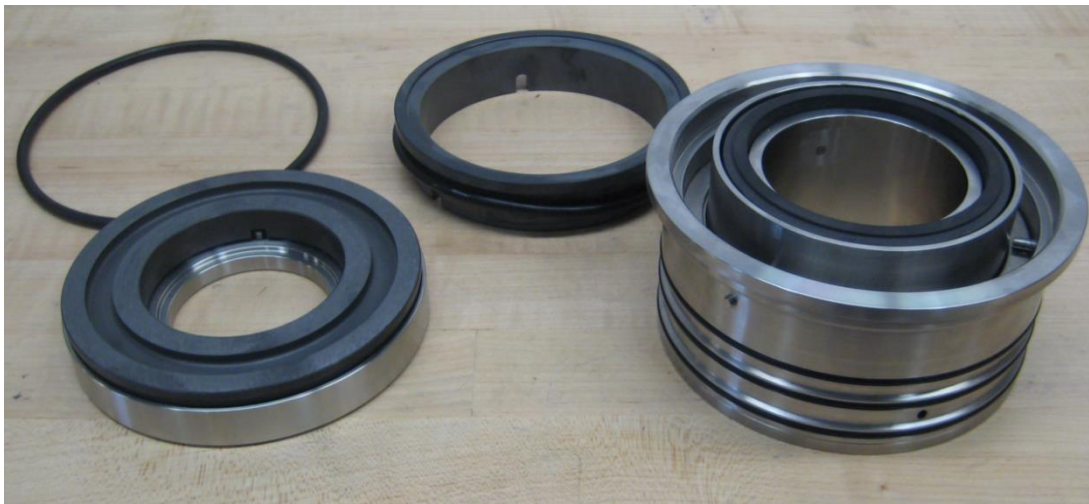
Figure 7.5-1: Various parts of the seal used in the CONTHERM MAX
