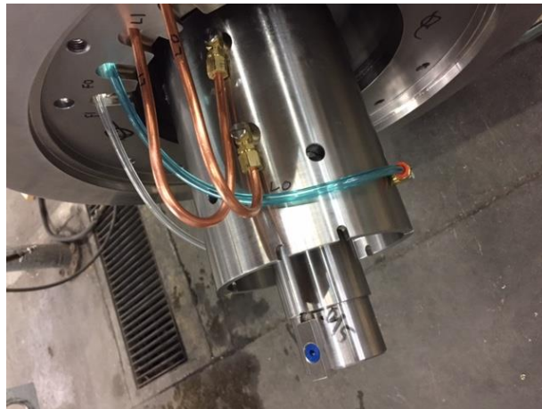
Figure 7.6-13: Attach the bucket assembly to the bearing housing
