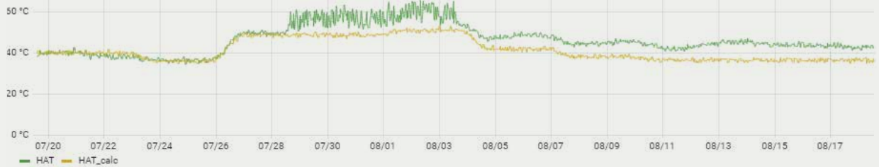
Fig. 2. By comparing the predicted and actual values, Packinox Performa can assess the condition of your Packinox heat exchanger.
