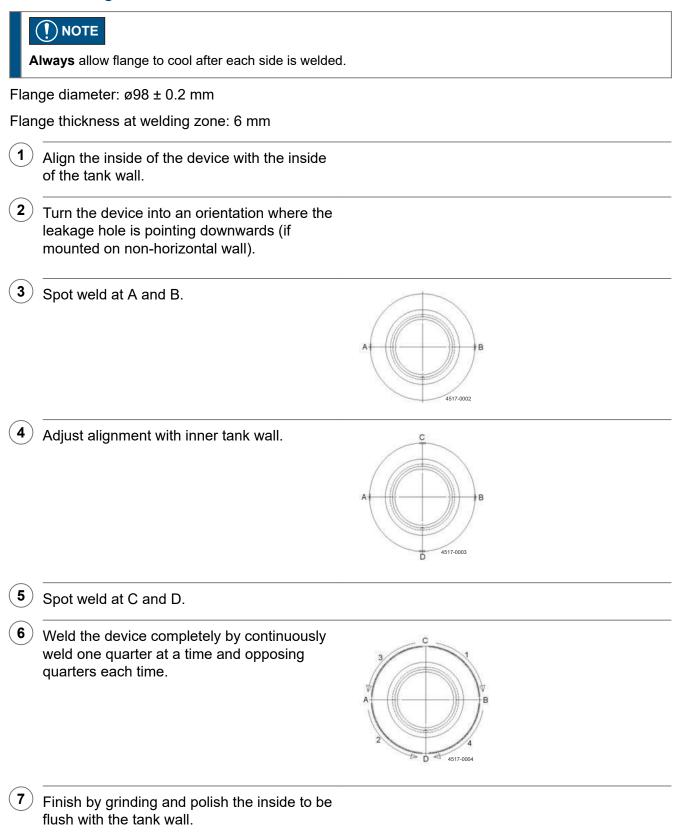
To ensure a hygienic weld it is recommended to either use shielding gas or pre-treat the welding zone to remove any discolouration.
