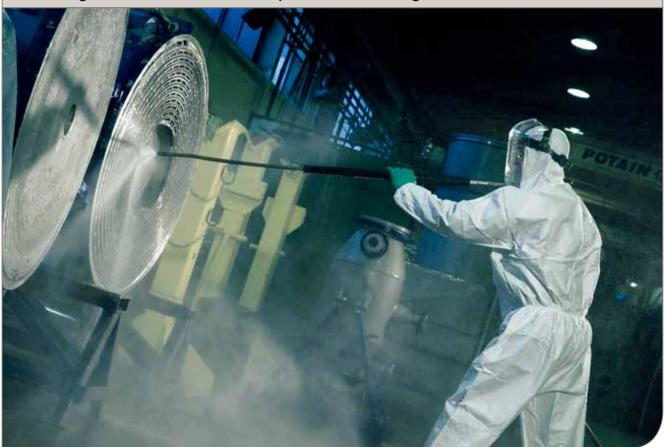
Alfa Laval spiral heat exchangers are the ultimate problem solvers. Their design prevents clogging and fouling in applications that other heat exchangers simply cannot handle. For the longest and most sustainable performance, however, even spiral heat exchangers require routine cleaning. Proper cleaning restores the optimal operating condition, ensuring maximum thermal efficiency, with lower maintenance costs and even a longer lifecycle for your unit.
