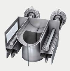
Alfa Laval's unique Spray Bar technology ensures effective mixing of the liquid feed and the recycle gas. The gas enters from the bottom and passes the Spray Bars, where the liquid feed is sprayed into the gas.
