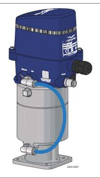
2 Verify that the air exhaust plug points downwards as indicated by the arrow to avoid water ingress in the pneumatic system. You can rotate the exhaust plug until it points in the right direction.
