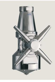
liquid in the tank. The nozzles rotate around both the horizontal and vertical axes in a 360° movement. This threedimensional jet rotation enables the jets to reach the entire tank volume, providing fast, efficient mixing of the injected liquid, gas or powder without requiring batch rotation.
