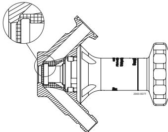
Manual valve: rotate the handle in a clockwise direction to close the valve. Pneumatic valve: shut the air supply to stop the flow of product from the valve. In closed position, the valve body is now ready for sterilization. If steam is used for Sterilization-in-Place, the use of an optional pressure relief valve on the outlet is recommended to ensure proper steam temperature in the valve.
