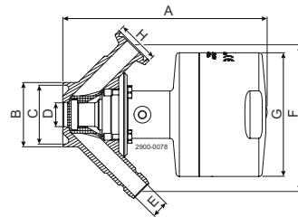
Figure 2. Pneumatic with valve body: Collared pipe welding
