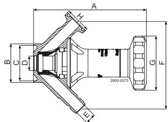
Figure 1. Handle with valve body: Collared pipe welding
