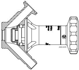
Manual valve: rotate the handle in a counterclockwise direction to open the valve. Pneumatic valve: open the valve by activating the actuator. This retracts the valve stem and the membrane, which enables the product to flow freely through the open valve.
