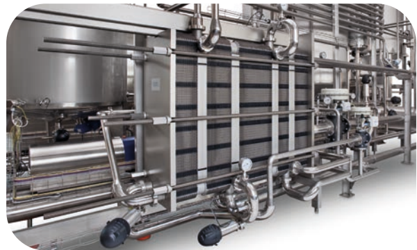
Alfa Laval FrontLine gasketed plate heat exchanger meets the highest demands on hygienic control and handling of heat-sensitive media.
