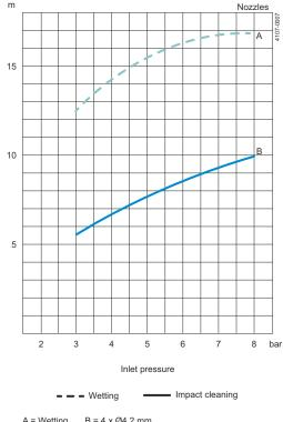
A = Wetting B = 4 x  $\varnothing$ 4.2 mm 4 x  $\varnothing$ 5.2 mm 4 x  $\varnothing$ 6.2 mm
