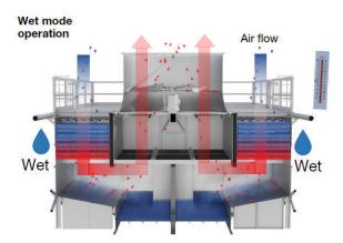
In cooler months, use **dry mode** (left). Air is pulled down over enhanced surface coils for cooling. In hotter months, use **wet mode** (right). Drenching water is sprayed over appropriately designed enhanced surface coils for increased cooling utilizing evaporative effect.
