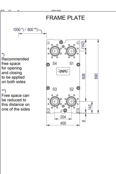
Space between pressure plate and supporting column should be kept free from fixed installations!
