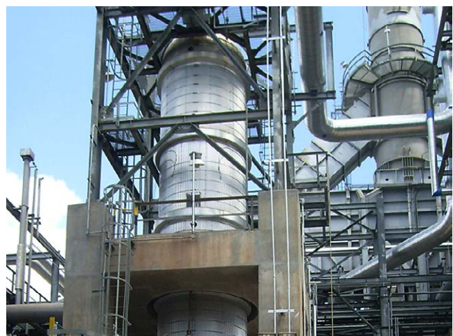
Alfa Laval Packinox combined feed/effluent heat exchanger installed in a petrochemical plant.
