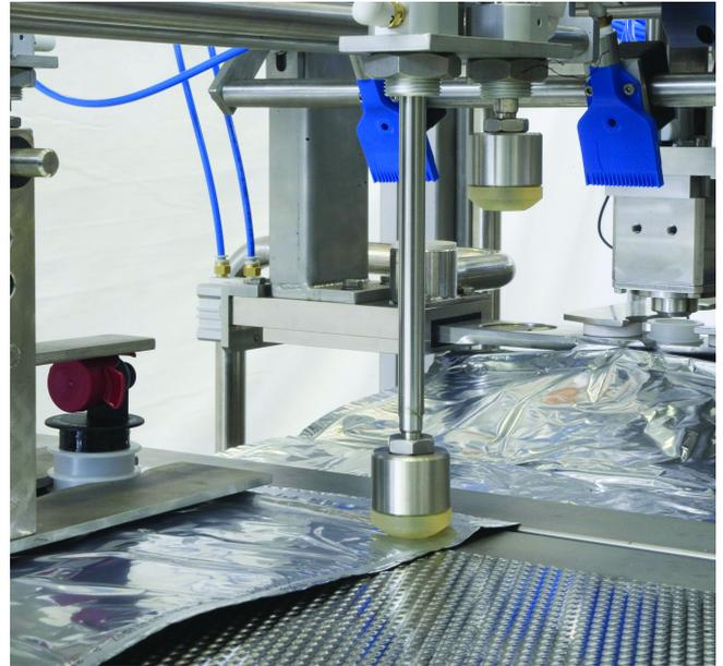
Detail: cap, horizontal bag separator, filling valve
