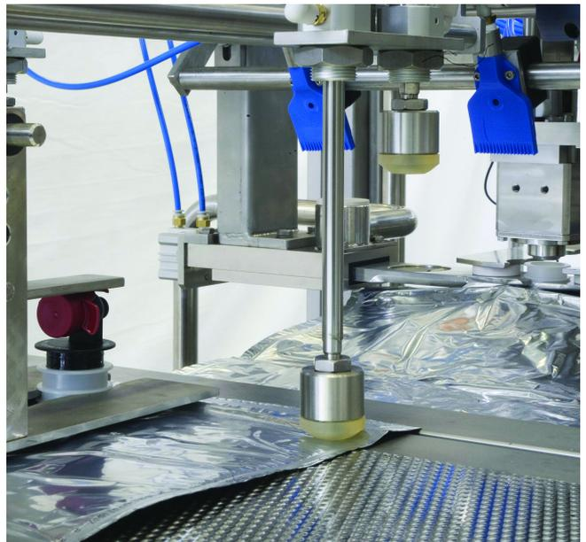
Detail: cap, horizontal bag separator, filling valve
