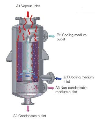
Minimal vapour pressure drop can be easily achieved, so that high-capacity vacuum systems are not needed. A large crossflow area within a short flow length allows the handling of large volume flows in a single unit.
