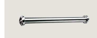
The mixer consists of an outer shell and an insert which is positioned at the centre. The insert is equipped with propeller shaped wings that puts the incoming liquid(s) into rotation. When this has been obtained, another pair of wings changes the rotation direction and the turbulence created gives an extremely effective mixing.
