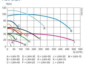
Frequency: 50 Hz Speed (synchr): 3000 rpm
