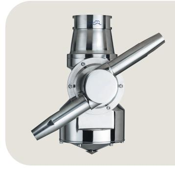
liquid in the tank. The nozzles rotate around both the horizontal and vertical axes in a 360° movement. This threedimensional jet rotation enables the jets to reach the entire tank volume, providing fast, efficient mixing of the injected liquid, gas or powder without requiring any batch rotation.
