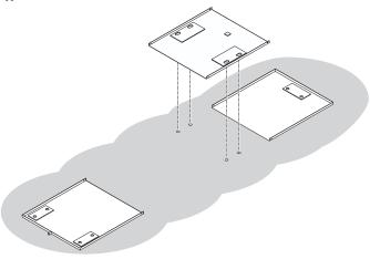
4 Put the connection tray in place. Fit the tray plates side by side.
