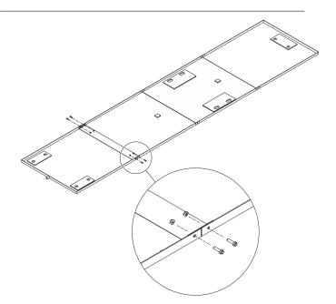
8 To prevent liquid leakage, apply polyurethane structural adhesive around the edges of each connection plate.
