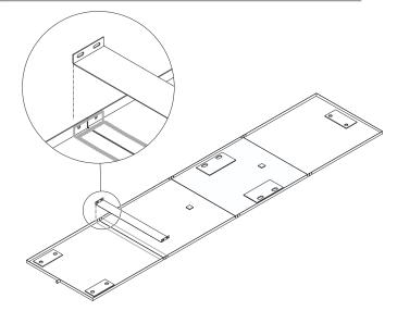
6 Put the connection plate in place. Fit it accordingly with the screw holes.
