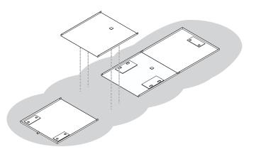
**5** To prevent liquid leakage, apply polyurethane structural adhesive under the connection plate.
