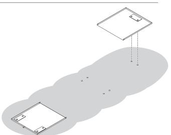
Put the tray below pressure plate in place. Align the support plate holes with the feet markings on the foundation.
