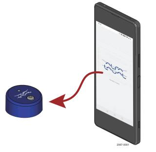
**2** Wake up the CM by shaking it, until the LED flashes blue or hold a magnet to the QR-code until the LED flashes blue, then remove the magnet.
